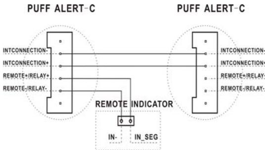
**Fig.2 Wiring of the Remote Indicator and/or interconnection**
