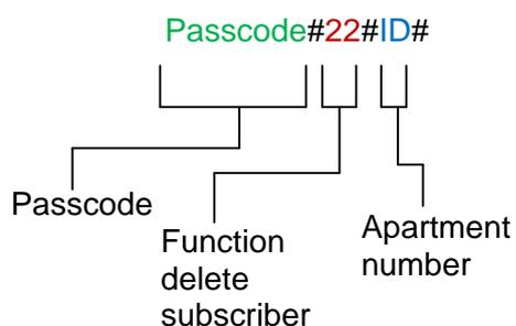
Additional SMS commands are shown below (SMS format assumes the standard default 123456 manager code has not been changed. If it has, replace this with the new code.
