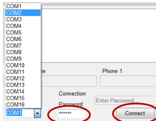
**TIP:** You may need to try this with several COM ports on your PC in order to find the exact COM port which is actually connected via USB to the intercom.
