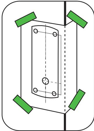
Diagram A - Drilling template taped to door
