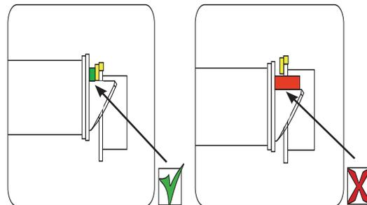
Diagram D - Strike plate position - Anti-shim plunger
