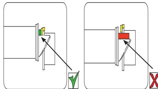
**Diagram D - Strike plate position - Anti-shim plunger**
