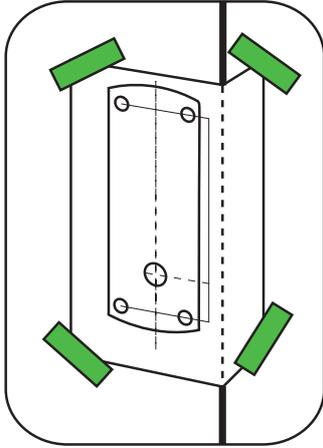
**Diagram A - Drilling template taped to door**
