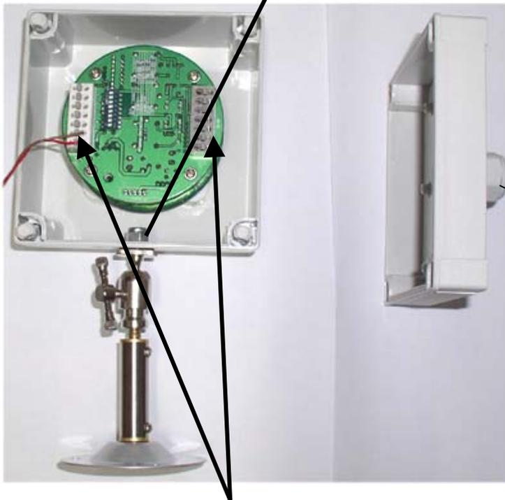
□ Separate the supplied cable gland/its nut and combine them to the Rear housing tightly.
